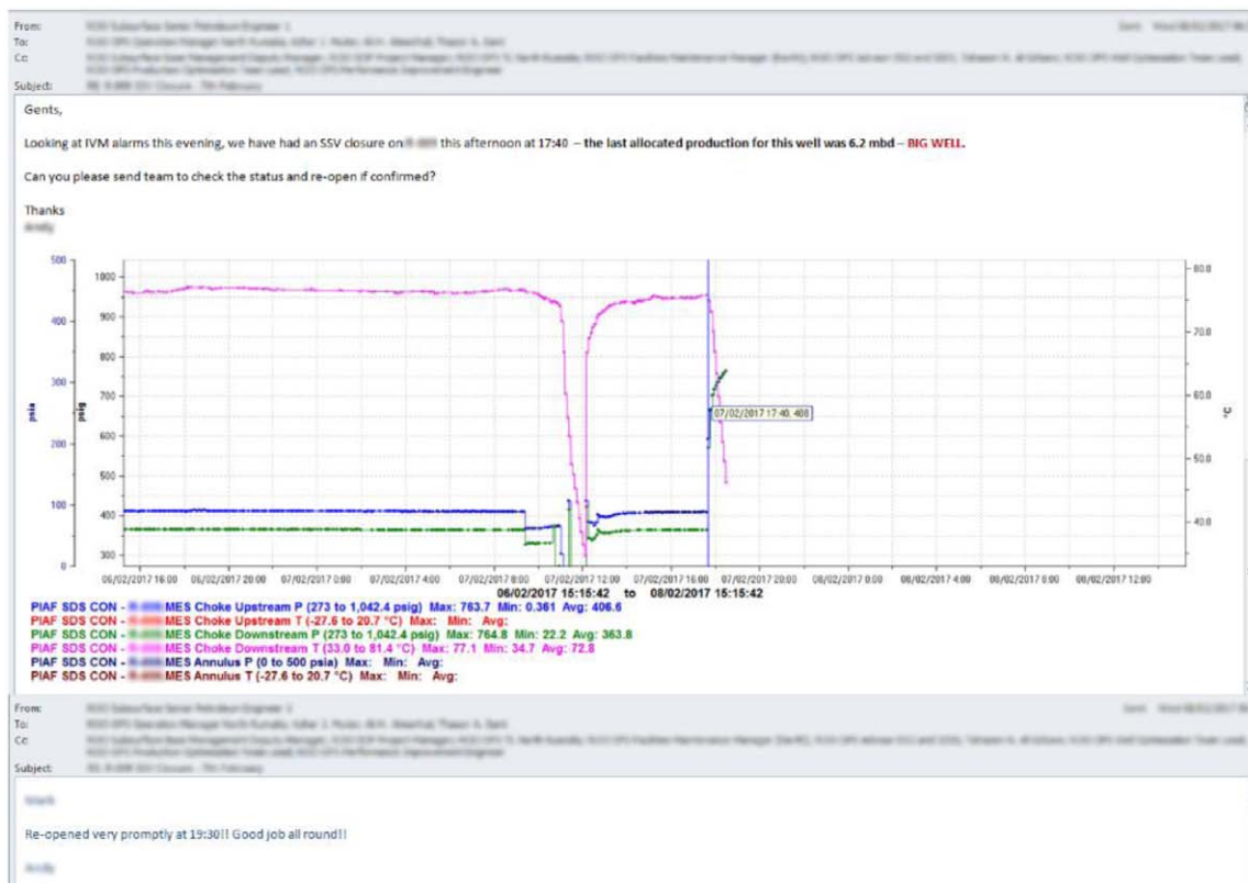
Figure 11—Real example of restoring production in less than 2hrs.
